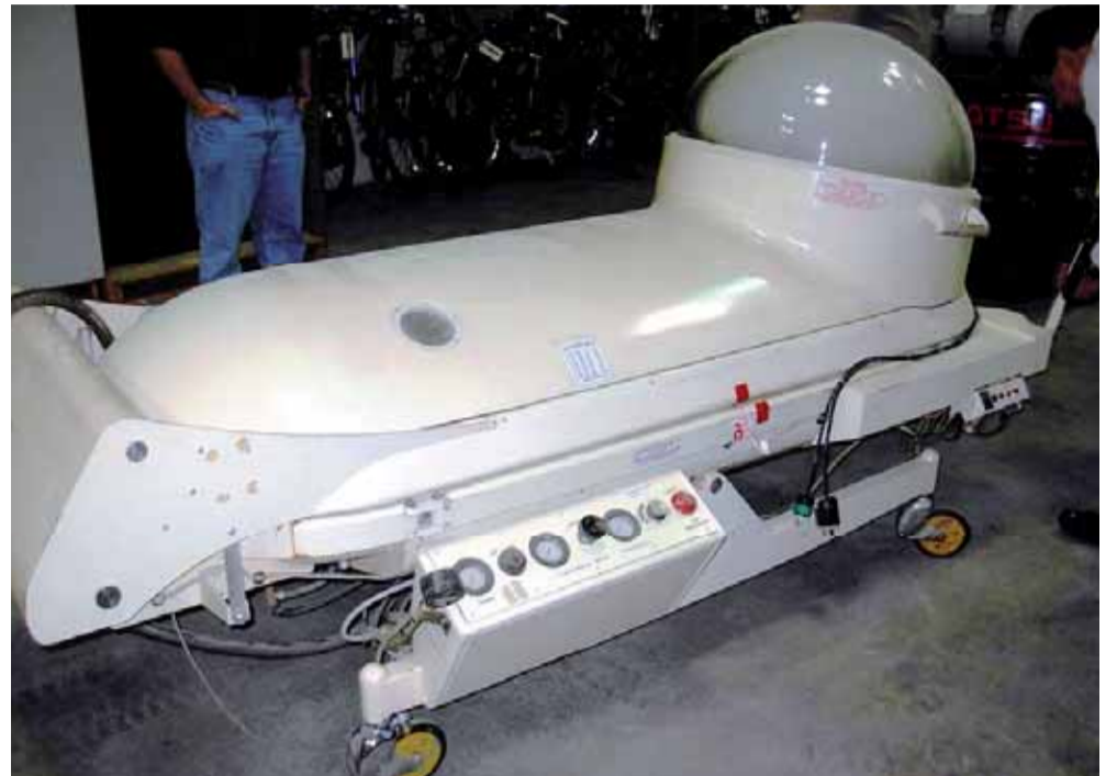
Exterior of Vickers 'clamshell' chamber with lid closed.
